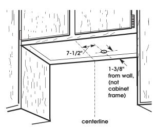
To wire through top, mark a line 7-1/2" from the right of the centerline on the underside of the cabinet. Mark the point on this line that is 1-3/8" from the back wall. Drill a 1-1/4" diameter hole through cabinet at this point. Note: If a cordconnection kit is used, drill a 1-5/8" diameter hole.
